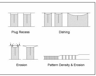
of recess due to the wet etching action of the slurry.
