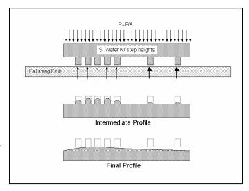
This pattern density effect on removal rate can cause problems if you have very dense and very sparse pattern in your design. Some ways to account for this is to create dummy shapes around the sparse pattern to try and match the higher pattern density.
