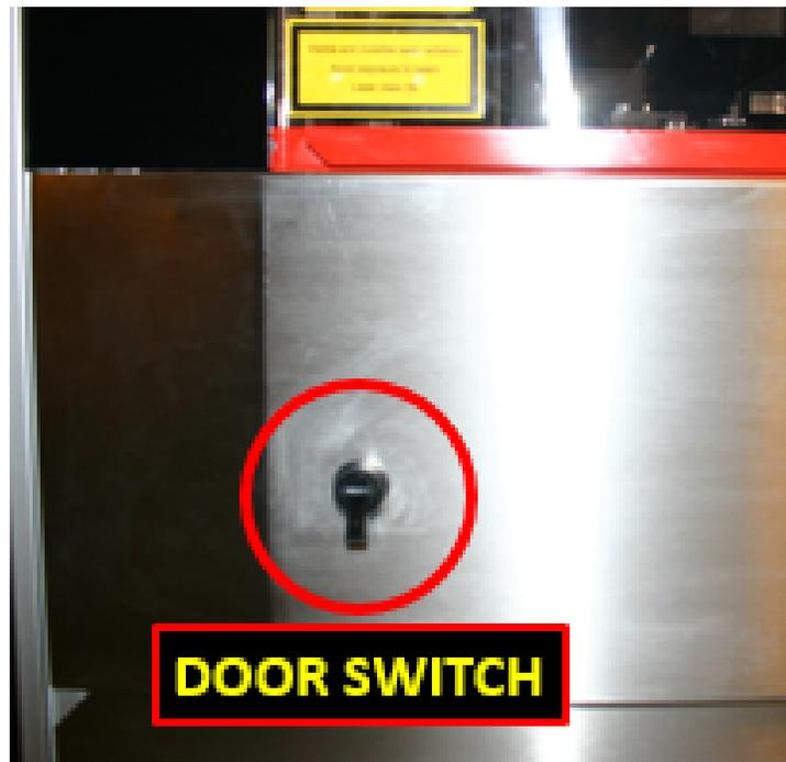
**NOTE:** When the main chamber door is open, the interlock disables any stage motion. Don't try to move, initialize, or home the stage with the door open.
