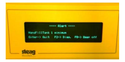
When the chemical level is low, a sensor signals the tool and an error message is displayed, such as "Handfill tank 1 minimum". The process will complete normally, but the tool will not begin a new cycle until the tank is refilled.
