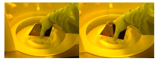
The Hamatech HMP 900 is a chemical spray-processing tool. The mask is spun to distribute chemical, then spun again to rinse and dry the surface. Both the front and back of the mask are rinsed with DI water.
