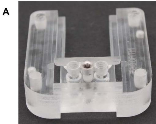
Figure 7; A: Low volume flow cell manifold (NTA0065 )
