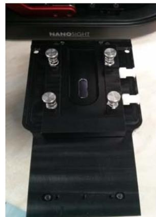
**Figure 20: Laser module with O-Ring top-plate unmounted from the NS300**
