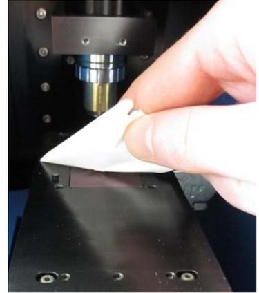
Figure 22: Cleaning the optical flat on the laser module
