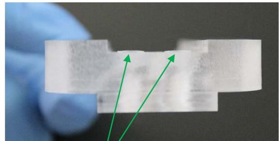
**Figure 15: Circular seals pressed fully down into the manifold (only just protruding from the surface)**
