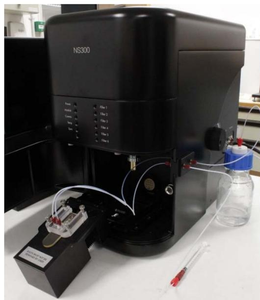
**Figure 9: Loading a sample with the low volume flow cell**
