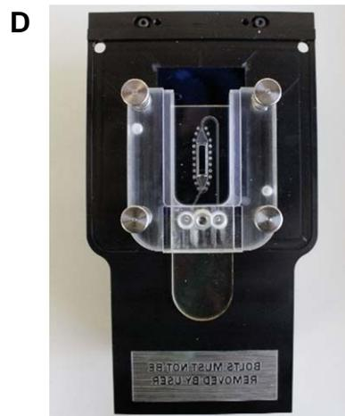
D: LVFC assembly mounted on laser module with sprung fastening bolts
