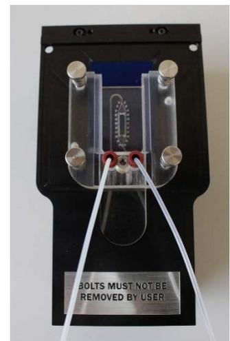
Figure 4: Low Volume Flow Cell
