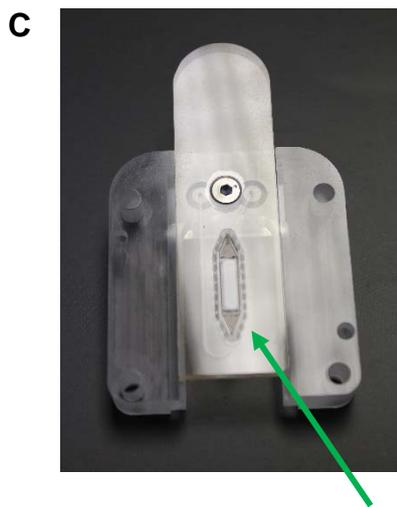
C: LVFC assembly with PDMS chamber seal on the underside of the gasket component
