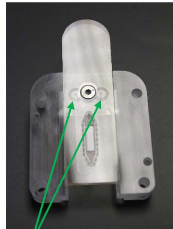
**Figure 16: Visual of the circular seal contact areas from underneath, confirming a good connection of the gasket component to the manifold**
