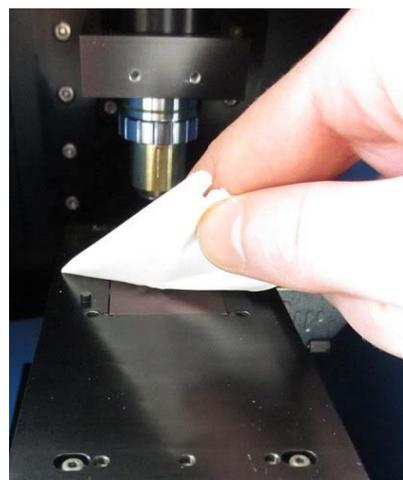
**Figure 11: Cleaning the optical flat on the laser module**
