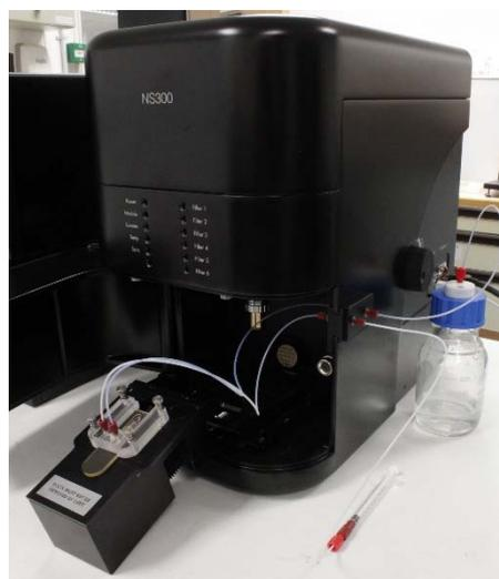
**Figure 8: Low Volume Flow Cell Tubing Configuration**
