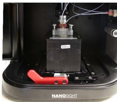
**Figure 10: Unmounting the laser module from the NS300**
