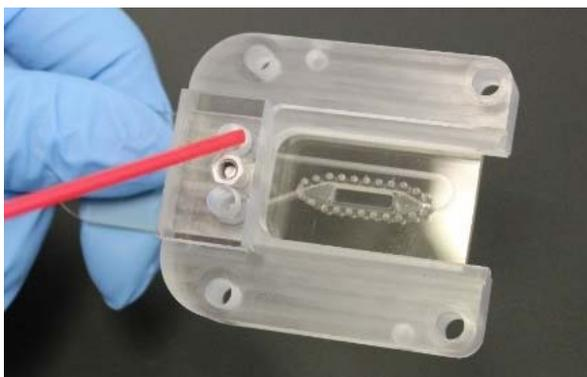
**Figure 13, A: Drying gasket component through manifold tubing ports**
