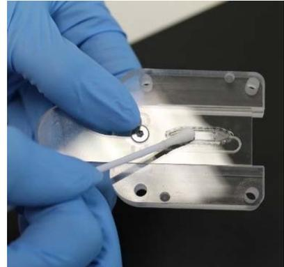
**Figure 12: Cleaning the underside of the glass window in the gasket component**
