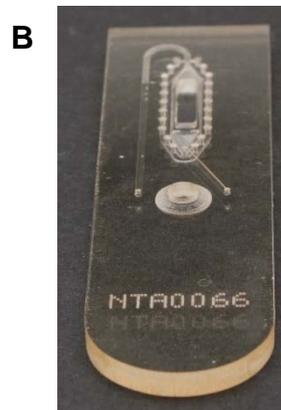
B: Low volume flow cell gasket component (NTA0066)
