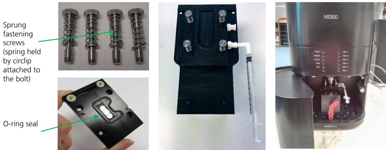
Figure 17; A Sprung fastening bolts and O-Ring Top-plate (ORTP)
