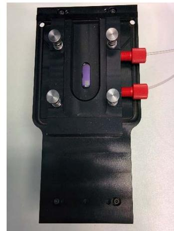
Figure 18: O-ring Top-Plate with tubing fittings for syringe pump use
