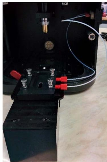
Figure 19: O-Ring Top-Plate Syringe Pump Tubing Configuration
