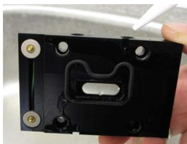
**Figure 21: Cleaning the O-Ring Top-plate**
