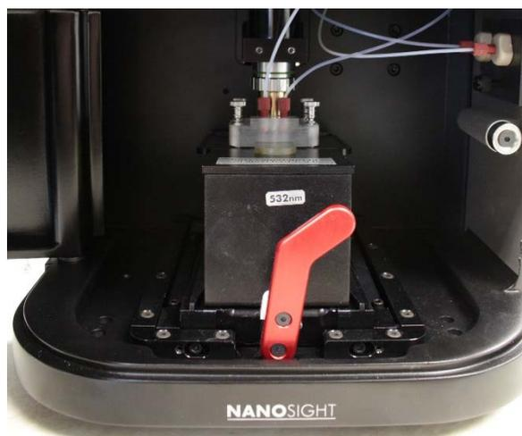
B: Laser module locked in position
